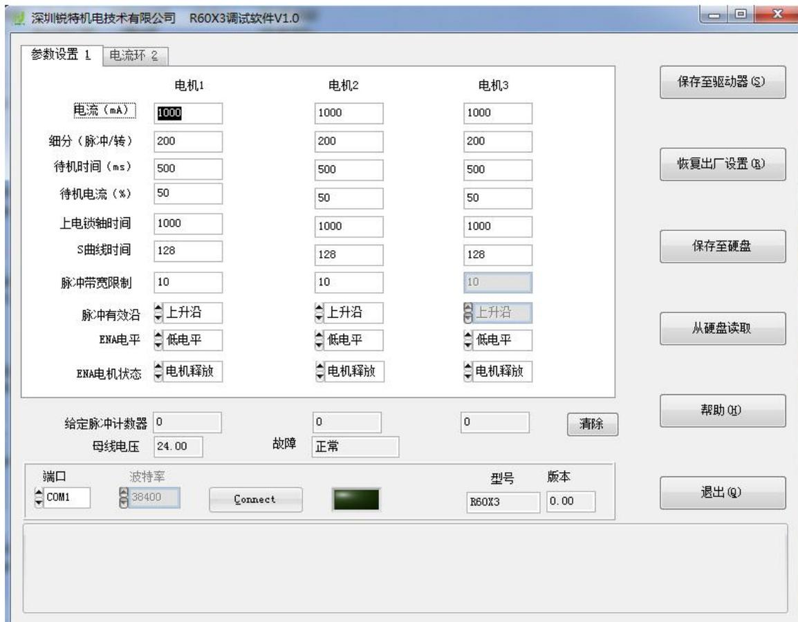
The three axis related parameters are independent and can be set separately as needed.
